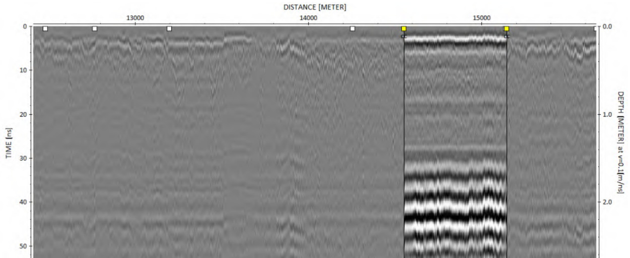
Figure 5.1: 400MHz Frequency – A high amplitude response occurring at a depth of c.0.12mbelow ground level (bgl) between chainage 14550 and 15150 indicates the presence of rebar in the pavement construction.
