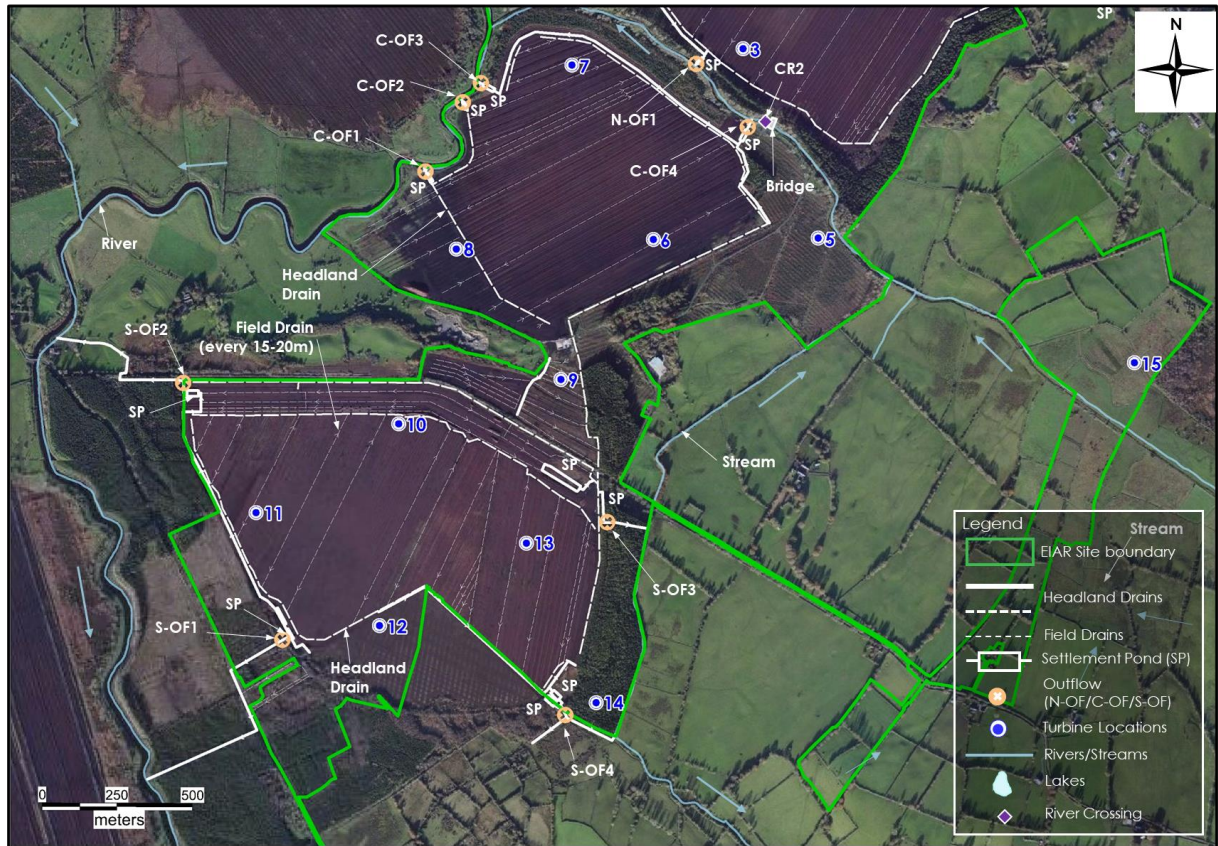
Figure A: Southern Basin existing drainage network
